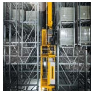
Stacker crane for pallets: speed and precision during storage and retrieval process.
