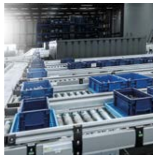
Case conveyor system for transporting products in boxes, containers and trays weighing up to 50 kg.
