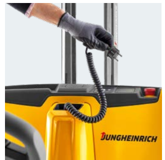
Ready to use again in no time: the integrated charger allows recharging at any 230 V socket.
